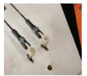
7 Easy Clevis Keepers If a clevis were to pop off one of your model's control horns, you could lose control and crash. A simple and cheap way to prevent this from happening is to add a clevis keeper. Simply slice a thin section from some model fuel tubing and slip it over the clevis. It will act like an O-ring and keep the clevis securely in place without binding.
